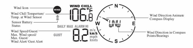
**Note**: The wind speed alert is set at 5 mph default and the wind gust alert is set to 7 mph default to prevent false alerts from small fluctuations.
