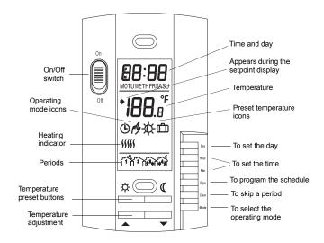
\* Set the switch to Off to cut power to the heater. This will not affect the time and temperature settings.
