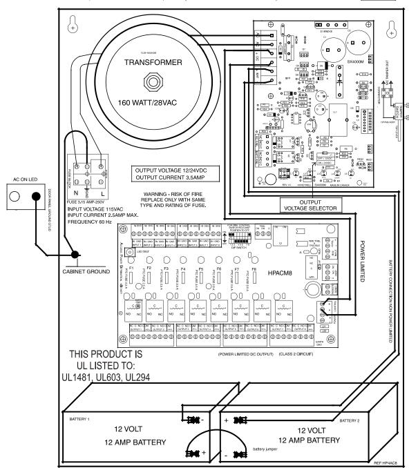
KEEP POWER LIMITED WIRING AT .25" MINIMUM SPACING
