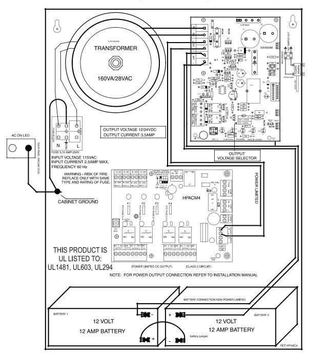
KEEP POWER LIMITED WIRING AT .25" MINIMUM SPACING FROM NON-POWER LIMITED
