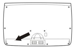
If the vent hole is covered by an object, e.g. a tracking label, other than an approved main battery, the touch screen may be damaged. Contact Technical Assistance if damage occurs for the process to follow when returning the device to Honeywell for repair.
