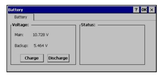
The backup battery draws power from the Main battery to maintain a charge. The backup battery voltage and percentage of power fluctuate continuously.
