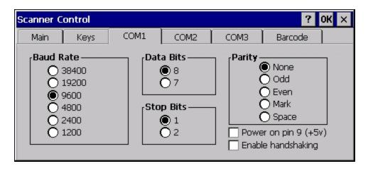
This panel sets communication parameters for any device connected to the external port. The settings for COM1 port on the MX3-RFID are pre-set and dimmed. Settings cannot be changed by the end-user. Baud rate is 115200, 8 data bits, 1 stop bit, no parity and power on Pin 9 is enabled.
