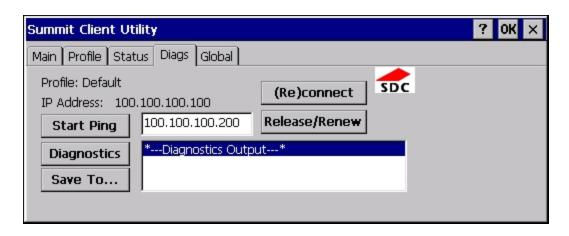
The Diags screen can be used for troubleshooting network traffic and radio connectivity issues.
