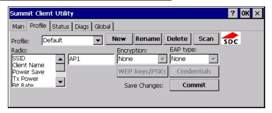
When logged in as an Admin (see Admin Login), use the Profile tab to manage profiles. When not logged in as an Admin, the parameters can be viewed, and cannot be changed. The buttons on this tab are dimmed if the user is not logged in as Admin. The Profile tab was previously labeled Config.
