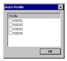
The Auto Profile selection screen displays all currently configured profiles. Click on the checkbox for any profiles that are to be included in Auto Profile selection then click ok to save.
