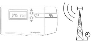
The ATS module picks up a daily time signal from a transmitter in Central Europe and corrects the time on the CCM61NG display. So:
