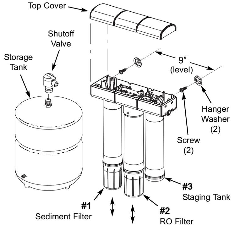
**NOTE:** Be sure to allow a minimum space of 1-1/2" under the system for removing and replacing the filters.
