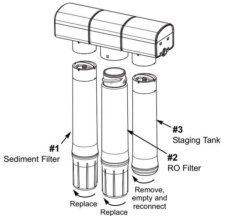
Turn cartridges in the direction of the arrow to remove. Turn them in the opposite direction to install.
