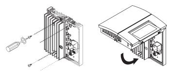
NOTE: If necessary, before re-installing the front component, configure the thermostat (see section 3).
