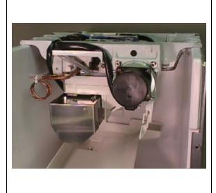
Unlike the initial harvest, the normal harvest is controlled by the thermistor. When the thermistor reaches 59°F, the control board deenergizes the hot gas valve and energizes the condenser fan motor. The actuator motor energizes to raise the plate. When the plate reaches the evaporator, the actuator toggle switch is moved back to the right. The board de-energizes the inlet water valve and the freeze cycle begins again. The average harvest cycle is about 3 minutes.
