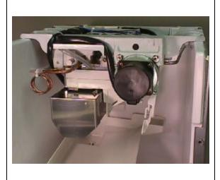
When the plate reaches the evaporator, the cam arm switch lever moves the actuator toggle switch to the right position. This stops the actuator motor and sets up the circuit to lower the plate in the next harvest cycle. It also energizes the pump motor and the board de-energizes the inlet water valve. The Freeze Cycle now begins.
