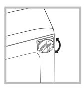
2. If the floor is uneven, the front feet of the machine may be adjusted until it reaches a horizontal position (the angle of inclination must not exceed 2 degrees).
