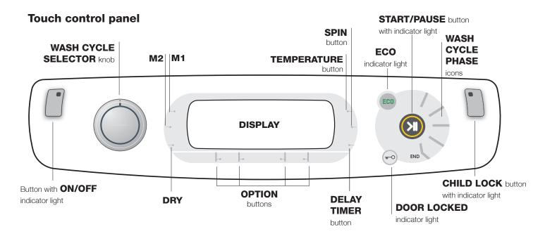
Button with (\*) **ON/OFF** indicator light: press this briefly to switch the machine on or off. The green indicator light indicates that the machine is switched on. To switch off the washer-dryer during the wash cycle, press and hold the button for approximately 3 seconds; if the button is pressed briefly or accidentally the machine will not switch off. If the machine is switched off during a wash cycle, this wash cycle will be cancelled.
