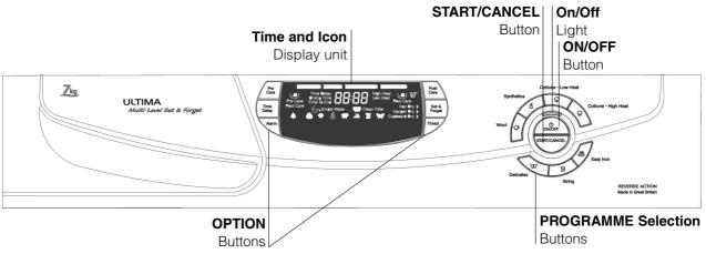
The **START/CANCEL** button starts a selected programme. When you press this button there will be one short beep and the progress icons will flash on/off to confirm the action. If you have not set a programme, the buzzer will beep four times. When a programme is running, holding this button in gives one long beep and cancels the programme and stops the dryer (*see Start and Programmes*).
