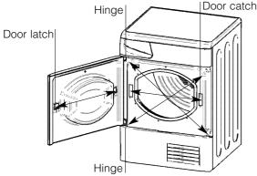
The door of your dryer is reversible and can easily be changed. Exchange diagonally hinge brackets and blanking screws. Exchange door latch and catch with their opposite blanking plates (*see diagram above*).
