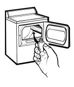
Before replacing the light bulb, be sure to unplug the dryer power cord or disconnect the dryer at the household distribution panel by removing the fuse or switching off the circuit breaker. Reach above dryer opening from inside the drum. Remove the bulb and replace with the same size bulb.
