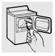
Before replacing the light bulb, be sure to unplug the dryer power cord or disconnect the dryer at the household distribution panel by removing the fuse or switching off the circuit breaker. Reach above dryer opening from inside the drum. Remove the bulb and replace with the same size bulb.
