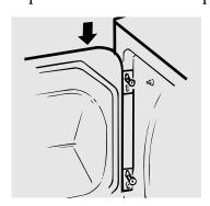
**7** Remove the remaining screws from the side of the opening from which the door was removed. With these screws secure each hinge at the bottom.
