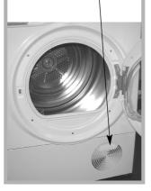
**STEP 2.** Remove the condenser by rotating the 3 clips then pulling the condenser
