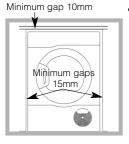
If you are going to install the appliance under a work counter, be sure to leave a 10mm space between the top and any other objects on or above the machine and a 15mm space between the sides and lateral furnishings or walls.
