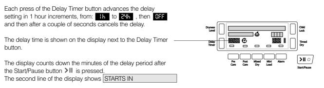
After the delay period finishes (or for all of the programme if delay not selected): The estimated Time to End of the programme for automatic programmes or the actual time remaining during the Timed programme is shown in this part of the display.
