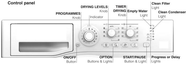
The **ON/OFF** button  $\bigcirc$ : If the dryer is running and this button is pressed and held for more that 3 seconds the dryer is turned off, the programme is then cancelled. Press and hold for more than 3 seconds and the dryer reactivates.
