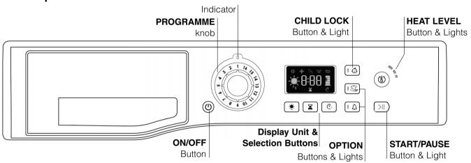
The **ON/OFF** button (1): If the dryer is running and this button is pressed and held for more that 3 seconds the dryer is turned off, it counts down 3, 2, 1, Off and the programme is then cancelled.
