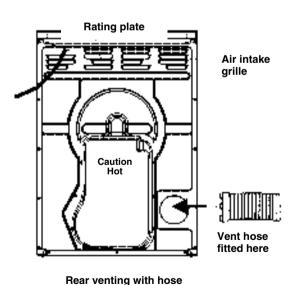
NOTE: When the dryer is in use, avoid touching the back of the machine as it may be hot.
