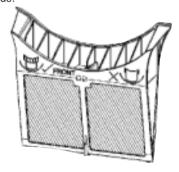
Wash or vacuum clean the filter occasionally. Don't be alarmed by the amount of fluff you may find on the filter. It's part of the wearing, washing and drying process.
