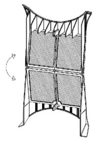
A very important part of your dryer is the fluff filter at the front edge of the drum. It's there to trap the particles of lint and fluff which are normally blown away when clothes are dried on the washing-line.
