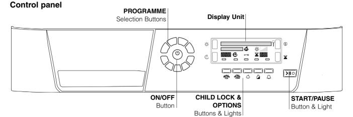
The **ON/OFF** button () - if pressed when the dryer is running: If the display shows TURNING OFF the dryer stops. If the display shows PRESS AND HOLD hold the botton and the display counts down 3, 2, 1 and then stops.
