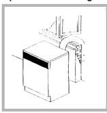
The end of the tube should be directed downwards, to prevent warm moist air from condensing in the room or in the dryer.
