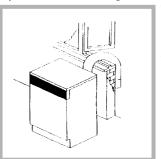
The end of the tube should be directed downwards, to prevent warm moist air from condensing in the room or in the dryer.
