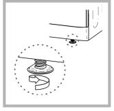
If the dryer is not level, use a wooden block to support it while adjusting the two front legs up or down, until your dryer is level.
