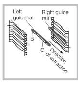
2. Choose which shelf to use with the sliding rack. Paying attention to the direction in which the sliding rack is to be extracted, position joint B and then joint C on the frame.
