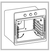
To assemble the sliding racks: 1. Remove the two frames, lifting them away from the spacers A (*see figure*).
