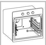
Secure the two frames with the guide rails using the holes provided on the oven walls (*see diagram*).
