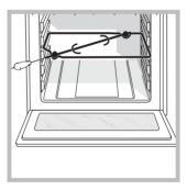
To operate the rotisserie function (*see diagram*) proceed as follows: 1. Place the dripping pan in position 1. 2. Place the rotisserie support in position 3 and insert the spit in the hole provided on the back panel of the oven.
