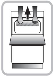
The cooker is designed to fit between kitchen cabinets spaced 500mm apart. The space either side need only be sufficient to allow withdrawal of the cooker for servicing. It can be used with cabinets one side or both as well as in a corner setting. It can also be used freestanding.
