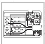
3. Remove the wire contact screws L-N---------, then fasten the wires under the screw heads, respecting the colour code: Black/Blue (N), Red/Brown (L) and Bare Wire/Yellow-Green (------).
