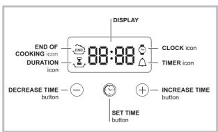
I The Top Oven and Main Oven can be controlled by the automatic timer. When the timer control has been set for one oven, it is possible to use the other oven only during the same automatic cooking programme.
