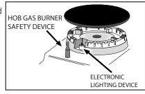
you must hold the control knob in for about 3-7 seconds after the burner has been lighted to allow the gas to pass until the safety thermocouple has heated.
