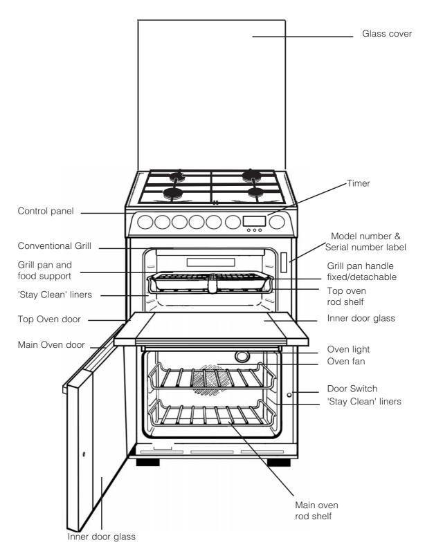
NOTE: To keep the controls cool when the appliance is used, a flow of air may be blown from beneath the control panel. If the appliance is still warm, this cooling fan will run on when all controls have been turned off. This is normal and is not a fault.
