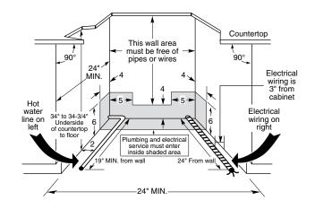
Note: Dishwasher must not be installed more than 10 feet from sink for proper drainage. All plumbing and electrical work must be in accordance with local codes. Dishwasher includes drain hose and leveling legs.
