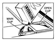
See "Detergent Usage Guide" below. (Be sure the Cycle Indicator Dial is at OFF position before adding detergent. Otherwise, the detergent cup will not close and *latch properly.*)
