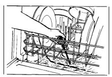
Remove the silverware basket and place a candy or meat thermometer in the water towards the middle of the tub. If the temperature is less than 120°F, you will not get good washing results. Higher water temperature is needed to dissolve grease and activate powder detergents.
