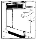
Special 1/4" thick wood inserts can replace the two metal panels. Dimensions for ¼" wood inserts: Door Panel: 23 ¼"W x 16¹¼6"H. Access Panel: 23 ¼"W x 6½"H.
