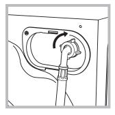
2. Connect the other end of the water inlet hose to the washing machine, screwing it onto the appliance's cold water inlet, situated on the top right-hand side on the rear of the ap-
