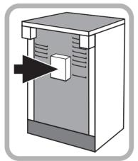
The control unit should be easily accessible in the event of an emergency, but must be within 2 metres of and not directly above an appliance.
