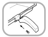
Replace screw and washers and ensure that they are fully tightened up. For a detachable handle remove screw and washers from grill pan and discard.
