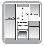
The height of the cooker can be adjusted by means of adjustable feet in the plinth (900mm - 915mm). Adjust the feet by tilting the cooker from the side. Then install the product into position.
