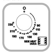
With the oven door closed, heating of the oven is achieved by turning the control clockwise to the required 'oven temperature' scale on the control panel, as recommended in the temperature charts. The pilot light will immediately come on and go off during cooking as the thermostat maintains the correct temperature.
