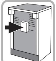
The control unit should be easily accessible in the event of an emergency, but must be within 2 metres of and not directly above an appliance.
