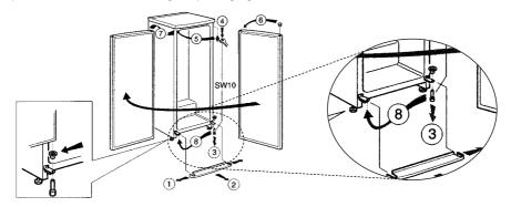
Insert the open door into the door bearing (A) IMPORTANT: The door journal (B) must be in front of the door switch (C)
