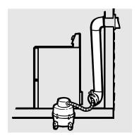
Inspect and clean the dryer exhaust ducting at least once a year to prevent clogging. A partially clogged exhaust can lengthen the drying time.
