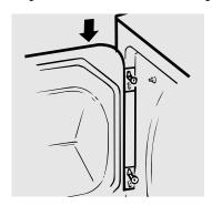
7 Remove the remaining screws from the side of the opening from which the door was removed. With these screws secure each hinge at the bottom.
