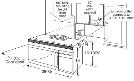
**Important Information:** When installing the Counter Saver Plus microwave oven over a range, allow minimum of 2" from bottom of Counter Saver Plus microwave oven to top of range backguard to allow for removal of light covers.
