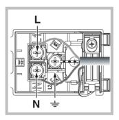
1. Open the terminal board by inserting a screwdriver into the side tabs of the cover. Use the screwdriver as a lever by pushing it down to open the cover (see diagram). 2. Install the power supply cable by loosening the cable clamp screw and the three wire contact screws L-N-Connect the wires to the corresponding terminals: the Blue wire to the terminal marked (N), the Brown wire to the terminal marked (L) and the Yellow/Green wire to the terminal
