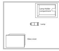
1. Remove the glass cover of the lamp-holder. 2. Remove the light bulb and replace it with a similar one: halogen lamp voltage 230 V, wattage 25 W, cap G 9.
