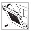
3. Grip the door on the two outer sides and close it approximately half way. Pull the door towards you, lifting it out of its slot (*see diagram*). To replace the door, reverse this sequence.
