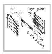
2. Choose which shelf to use with the sliding rack. Paying attention to the direction in which the sliding rack is to be extracted, position joint B and then joint C on the frame.
