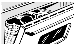
Leave the door open to the broil stop position. The door stays open by itself, yet the proper temperature is maintained in the oven.
