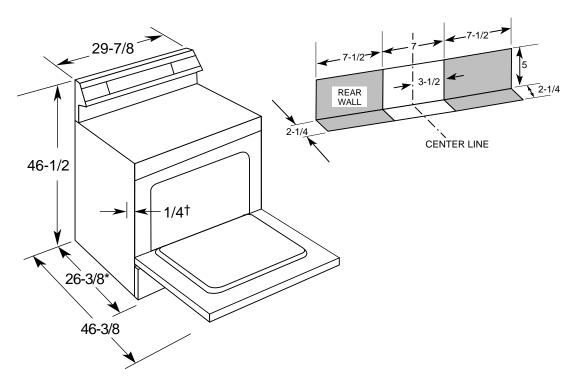
\*Dimensions from wall to front of closed oven door. Dimensions from wall to front of closed oven door handle is 28-3/8".
