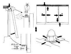
Adjusting the base. Cut out the plinth of the cabinet to match the aplliance bottom ventilation grille.
