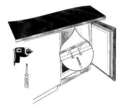
Mounting the kitchen cabinet door. Remove the top bracket from the appliance and secure to the door panel.
