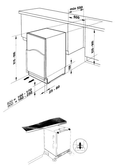
Make sure that the appliance is sitting level on the floor by adjusting all four feet.
