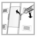
Access the light bulb as shown (*see diagram*) and replace it with a similar light bulb, the power of which should not exceed 10 W.
