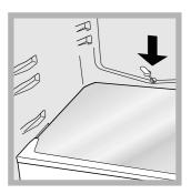
It is necessary to clean the discharge hole regularly so that the water can flow out easily. Do not use any tools that may damage the refrigerator.
