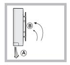
**AIR** maximises air circulation, improving the efficiency of the evaporator and helping to achieve the optimal temperature inside the refrigerator as quickly as possible each time it has been opened. The blown air (A) is cooled when it comes into contact with the cold wall, whereas the hotter air (B) is sucked up (see diagram).
