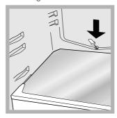
water is ducted to the back of the appliance by a special discharge outlet (see diagram) where the heat produced by the compressor causes it to evaporate. It is necessary to clean the discharge hole regularly so that the water can flow out easily.
