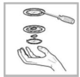
Remove the plug! Bulb/s: Remove the overhead light and remove the bulb to change. Only use 40W lamps. Make sure the bulbs are cold before touching them.
