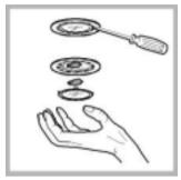
Remove the plug! Bulb/s: Remove the overhead light and remove the bulb to change. Only use 40W lamps. Make sure the bulbs are cold before touching them.
