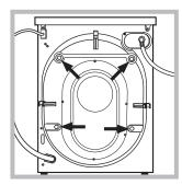
2. Remove the 4 protective screws (used during transportation) and the corresponding spacer, located on the rear part of the appliance (see figure).
