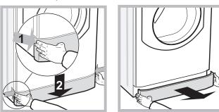
1. take off the cover panel on the front of the machine by first pressing it in the centre and then pushing downwards on both sides until you can remove it (see figures);
