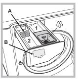
Loo not pour detergent into the compartment 1. Detergent should only be poured into the compartment 2.
