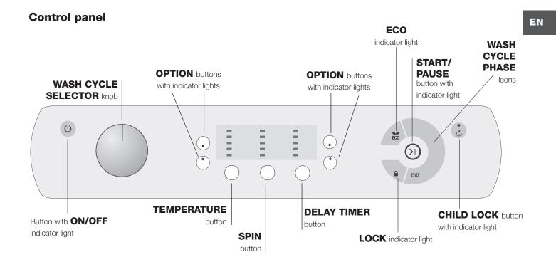
Button with () **ON/OFF** indicator light: press this briefly to switch the machine on or off. The green indicator light indicates that the machine is switched on. To switch off the washing machine during the wash cycle, press and hold the button for approximately 3 seconds; if the button is pressed briefly or accidentally the machine will not switch off. If the machine is switched off during a wash cycle, this wash cycle will be cancelled.
