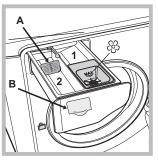
I Do not pour detergent into the compartment 1. Detergent should only be poured into the compartment 2.
